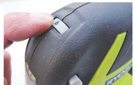
This top-mounted thumbwheel makes for easy speed control
